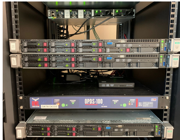
Defensive network design using data diode
