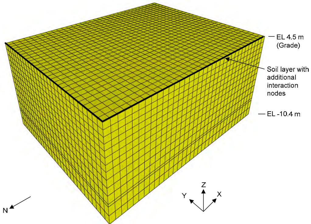
Figure 3: Excavated Soil-Rock Volume for CB MSM1 Model
