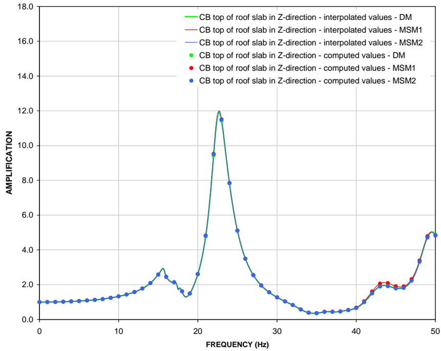
Figure 13: Z-Direction DM, MSM1, and MSM2 Transfer Functions CB top of roof slab (EL 13.8 m)
