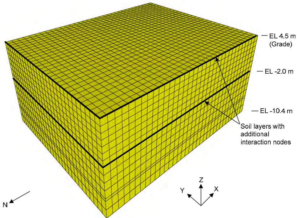
Figure 4: Excavated Soil-Rock Volume for CB MSM2 Model
