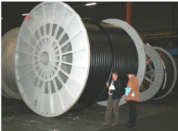
Factory Inspection of XLPE Cable
